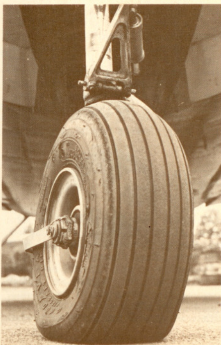
Underinflation causes tires to generate excessive heat on landing or takeoff which can lead to breakdown of cords and premature tire failure. It also results in hard to control ground characteristics.
