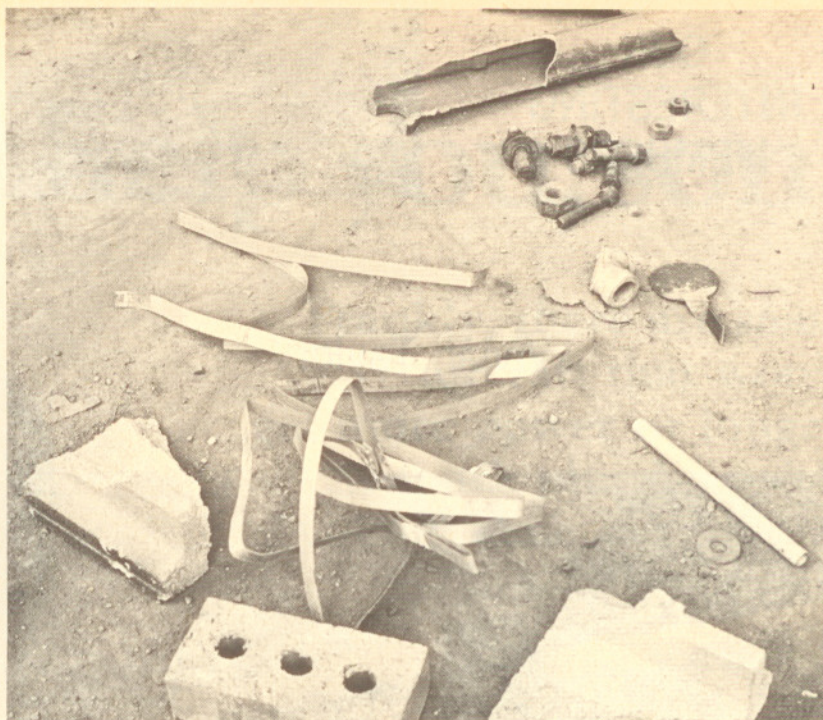
Some of the debris that must be avoided to insure longest service from your tires. All of these items were gathered from within the boundaries of an airport and any one of them could mean an abbreviated life for a lightplane tire.
